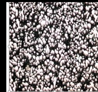
Slurry: Non-dendritic shear strength of about 0.2 kPa at fs=40%
