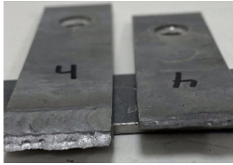
ENAB 42000 (Rheocasting) welded together Tensile testing
