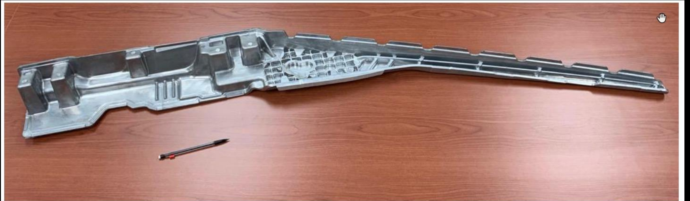
Figure 1- Hinge Pillar casting for large EV, produced in Comptech Rheocasting Process by Dynatool Industries Inc.
