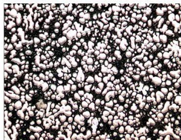
Slurry: Non-dendritic shear strength of about 0.2 kPa at f_s=40\%
